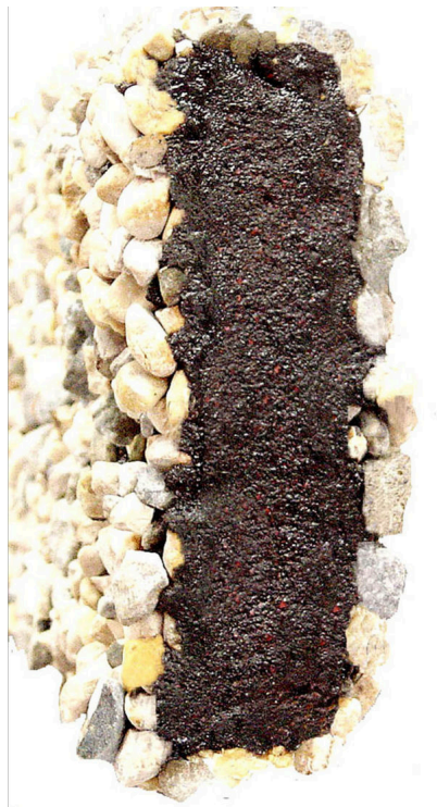
Incorporation of a band type R4 in the fresh concrete of the 1st concreting stage.
