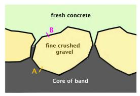
The core of BFL-Mastix waterstop is composed of a soft and deformable material, based on deformable elastomer rubber.
