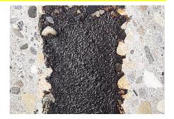
Water **cannot pass** around the BFL-Mastix waterstops. Water **cannot flow** along the waterstops.
