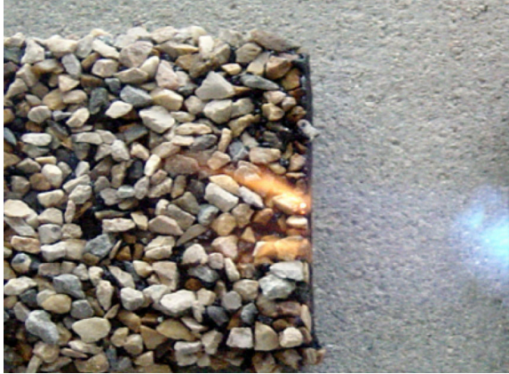
1 Flaming the contact surfaces
