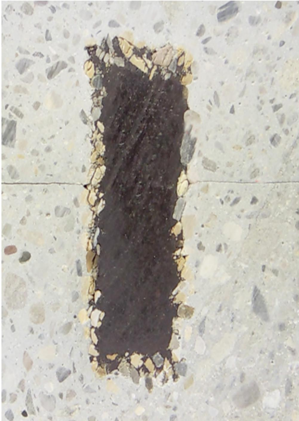
**BFL-Mastix waterstops consist of two components, a deformable bitumen/rubber core and a tightly anchored fine crushed gravel coating.**
